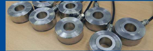
6x Load cells on the Main Bearing bolts
